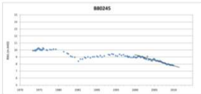
Figure 13a: Hydrograph from the Upper Tertiary Aquifer near Beaumaris (B0245) showing declining groundwater elevations, particularly since 2000.
